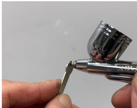
**Tighten the nozzle by hand until it seats (finger-tight).**
