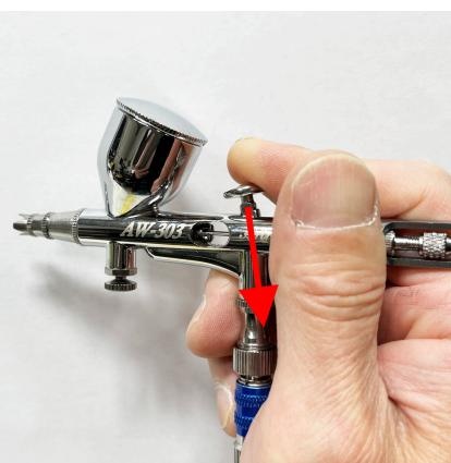
For beginners or those unfamiliar with using an airbrush, it is recommended to keep the trigger pressed down continuously during operation.
