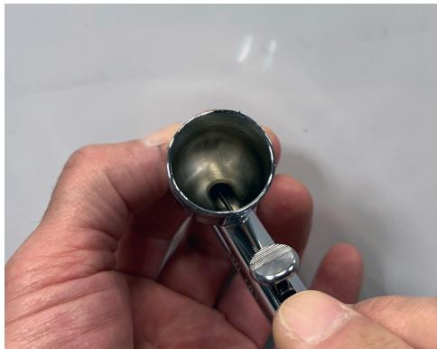
Finally, pour a small amount of thinner or cleaning solution into the airbrush again and backflush once more. If the liquid remains clear, it indicates that the inside of the airbrush has been thoroughly cleaned.
