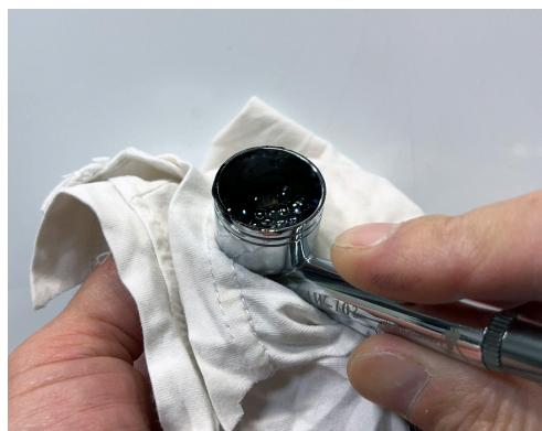
Pour a small amount of thinner or cleaning solution into the airbrush cup. Alternate between spraying and backflushing until the cleaning fluid runs clear, ensuring the inside of the airbrush is completely clean.
