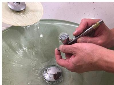
Reverse flush the airbrush until the water runs clear. However, reverse flow alone only moves air inside the nozzle, so alternate between spraying and backflushing to achieve a more thorough internal cleaning.
