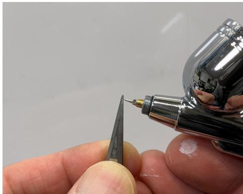
If the needle becomes bent, it can be temporarily straightened using tweezers or similar tools. However, this is only a short-term fix— even a slight bend will prevent the airbrush from producing fine lines, so replacement is recommended.
