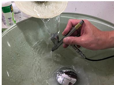
After using water-based paints, clean the airbrush by rinsing it thoroughly with tap water or by immersing it in a container of clean water.
