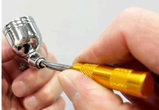
You can adjust the alignment using pliers or other tools, but the process is much easier with the **Nozzle Centering Tool** included in the **Airbrush Maintenance Kit**.
