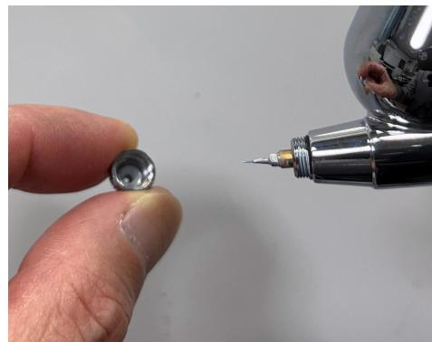
Remove the nozzle cap and check the tip. If you see any paint residue like in the image, cleaning is required.
