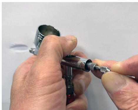
While releasing air, gently push the needle forward until the paint flow completely stops.
