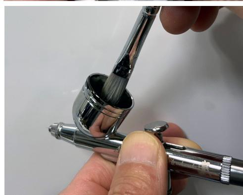
Use a cloth or a firm brush to clean any paint residue from the exterior surfaces of the airbrush.
