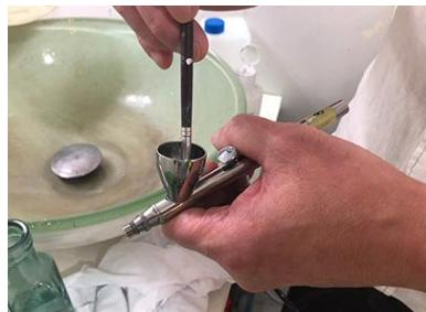
For areas where paint has dried or hardened, use cleaning solution and a firm brush (a flat pig-hair brush is recommended) to gently dissolve and remove the residue. This method helps keep the internal components of your airbrush clean and in optimal condition.
