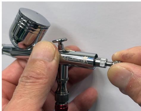
Remove the tail cap and slightly loosen the needle chucking nut.
