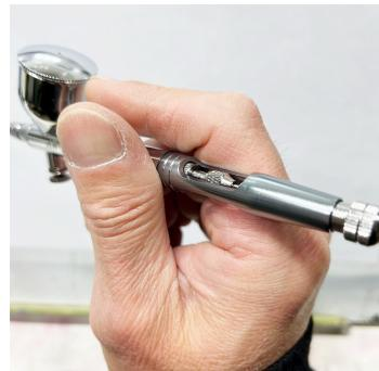
By rotating the tail cap up or down, you can change its position to prevent your finger from pressing into the opening.
